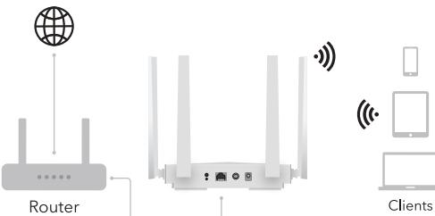
Connect wirelessly by using the default SSID printed on the bottom label of the product. Launch a web browser and enter <http://cudyap.net/> in the address bar. Create a password to log in.
